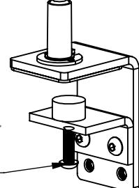
Fasten the screw for clamp tightening.
