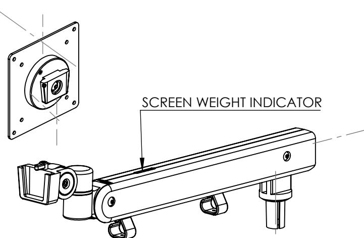
Please ensure the bush is placed with the slot aligned with the locking grub screw.
